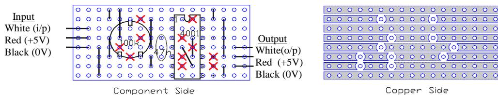
The circuit can be made up on a small scrap of Stripboard (Veroboard). The right hand sketch above shows where the tracks on the copper side must be cut using a 1/8" drill bit. Note the two wire links, which must be fitted first as they will be underneath the integrated circuit. The position of pin 1 of the ic is shown. The actual chip will either have a small hole adjacent to pin 1, or there will be a central notch at that end of the chip.
