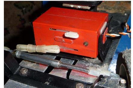
Linkages to servos may be push rods, push-pull Bowden cables (known as “Snakes”), or closed loop cables. The terminations for each of these will be similar.
