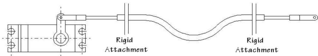
Because some clearance is required between the inner and outer so that the inner can slide freely, a small amount of backlash is inevitable when using a snake.
