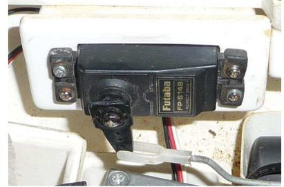
An alternative layout is the “Linear” servo. This has the advantage that the servo output has a fixed alignment, which is useful if the output shaft has to pass through a waterproofing seal.
